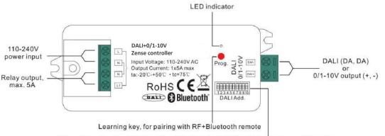
Dip switches to select DALI or 0/1-10V output, DALI DT6 or DT8 color type, DALI address or group control mode, DALI address to be controlled, DALI group to be controlled
